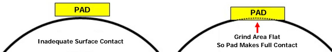
3. **Clean the sensor attachment pad.** Use a dry rag to clean the surface of the pad that will mate with the bearing housing. Sometimes the pads have residual machine oil that is left over from the manufacturing process used to create the pad.
