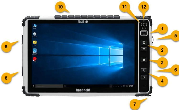
1. **Power:** Press and hold 4 seconds to turn on. When on, press again to put to sleep.
